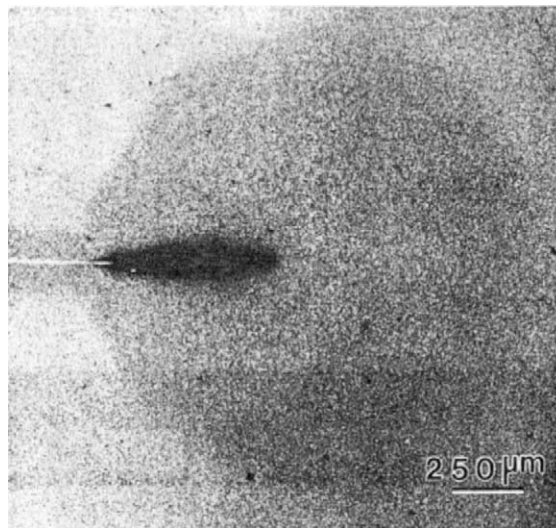
Fig. 6. Optical micrograph of a thin section taken at the mid-plane near the crack tip in the rubber-modified epoxy (from Pearson and Yee, 1991).
